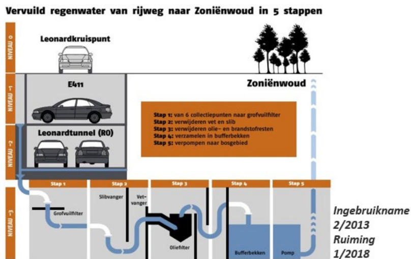
Figure 15: Technical water treatment system beneath the Leonard crossroad tunnel system receiving the runoff water from both the E411 and R0.
